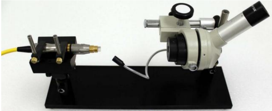
Figure 11-3 Optical fiber ends are fixed with the microscope
