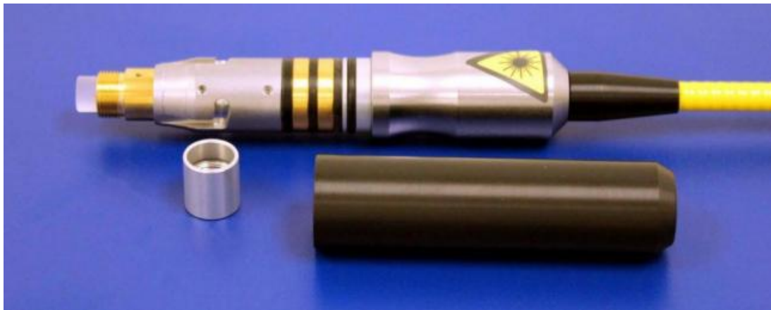
Figure 11-4 Remove the optical fiber protective cover and aluminum protective sleeve
