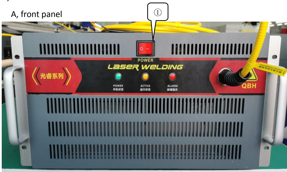
Figure 1-Physical picture of the front panel of the 3 / 150W laser
